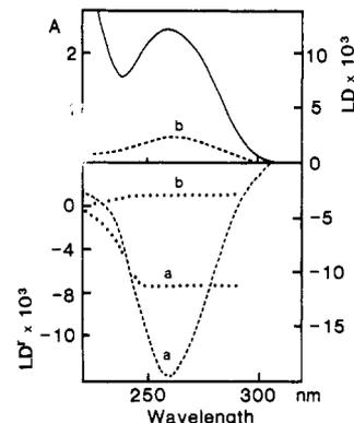
FIGURE 1: Absorbance [ $A$  (—)], linear dichroism [ $LD$  at a flow gradient  $G = 1800 \text{ s}^{-1}$  (- - -)] and reduced linear dichroism [ $LD^r$  (· · ·)] spectra of chromatin in 0.1 mM NaCl (a) and in 10 mM NaCl (b). The spectra are normalized to 1-cm optical path length.
