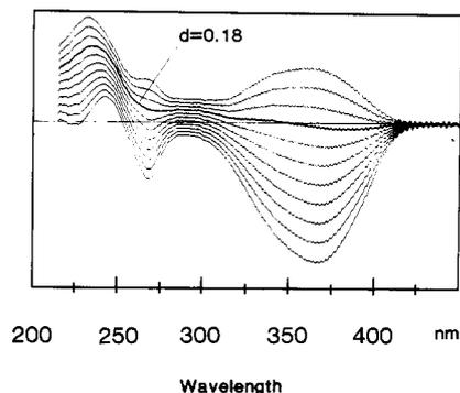
**Figure 5.** Linear combinations ( $A_{\perp} - dA_{\parallel}$ ) between the two polarized absorption spectra of DAPI in PVA film. The coefficient  $d$  is varied between 0 and 0.6 in steps of 0.06. The combination for which the feature at 260 nm disappears ( $d = 0.18$ ) is shown with bold line.
